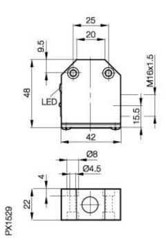
Inductive Sensors BES 516-344-H2-Y 22 x 42 x 48 normally-open Sn=5mm shielded
